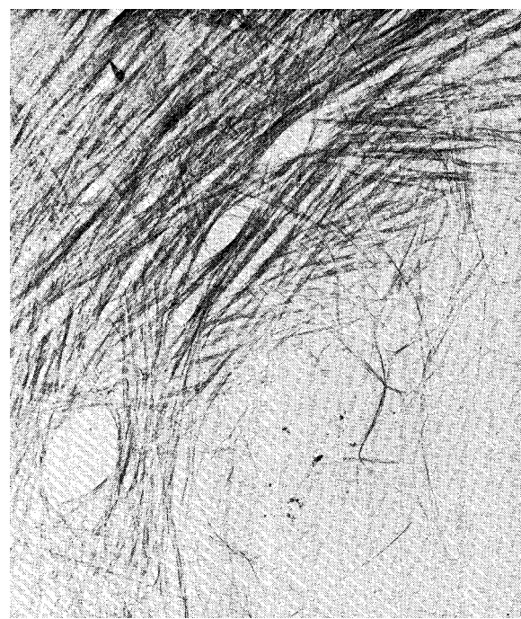
Fig. 12 Atactoid phase of a vanadium pentoxide dispersion (electron microscopy image) (reprinted with permission from J. H. Watson, W. Heller and W. Wojtowicz, Science , 1949, 109 , 274. Copyright 1949 American Association for the Advancement of Science. Readers may view, browse, and/or download this material for temporary copying purposes only, provided these uses are for noncommercial personal purposes. Except as provided by law, this material may not be further reproduced, distributed, transmitted, modified, adapted, performed, displayed, published or sold in whole or in part, without prior written permission from AAAS).
